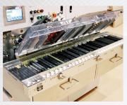
A consecutive process with automatic transportation system from Wet Blasting, rinsing to cutwater.
