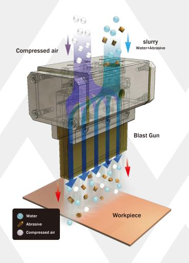
Wet blasting is a non-chemical etching method that accelerates slurry, which is a mixture of abrasive and water, with compressed air and projects it against the target object to process its surfaces.
