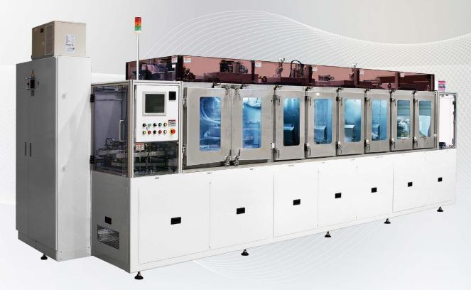
Automatic wet blast machine which processes cemented carbide chips (inserts) collectively for each tray, with two Wide quns.
