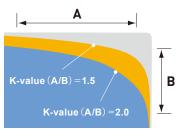
Cross-sectional view of cutting edge shape
