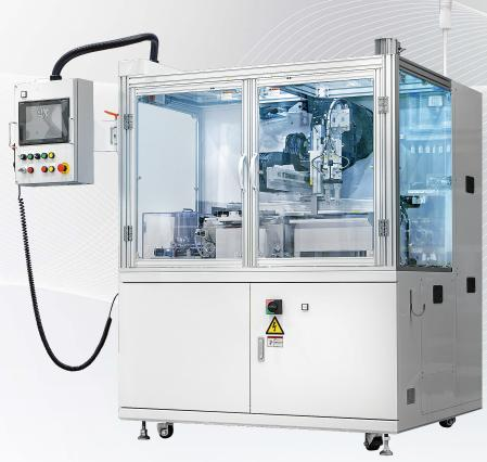
This wet blasting equipment is for cutting tools and processes each workpiece individually. The biggest feature is that it can achieve high-precision processing because the workpieces are handled individually and automatically processed one by one.
