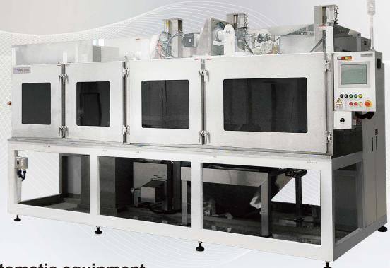
Automatic equipment that wet blasts the entire circumference of rod-shaped bar material evenly and at high speed.
